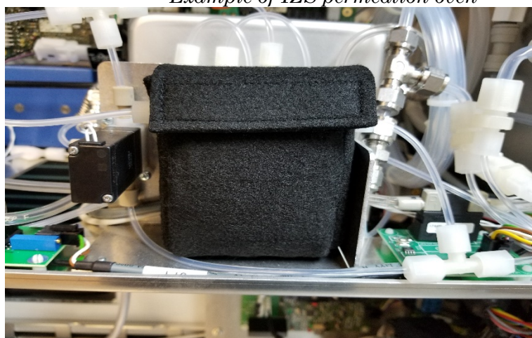
Example of IZS permeation oven
