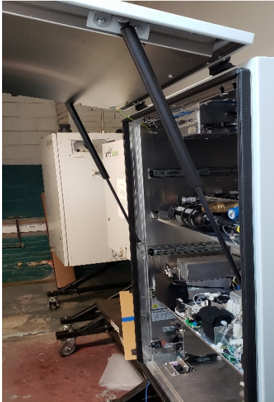
Gas shock and door seal
