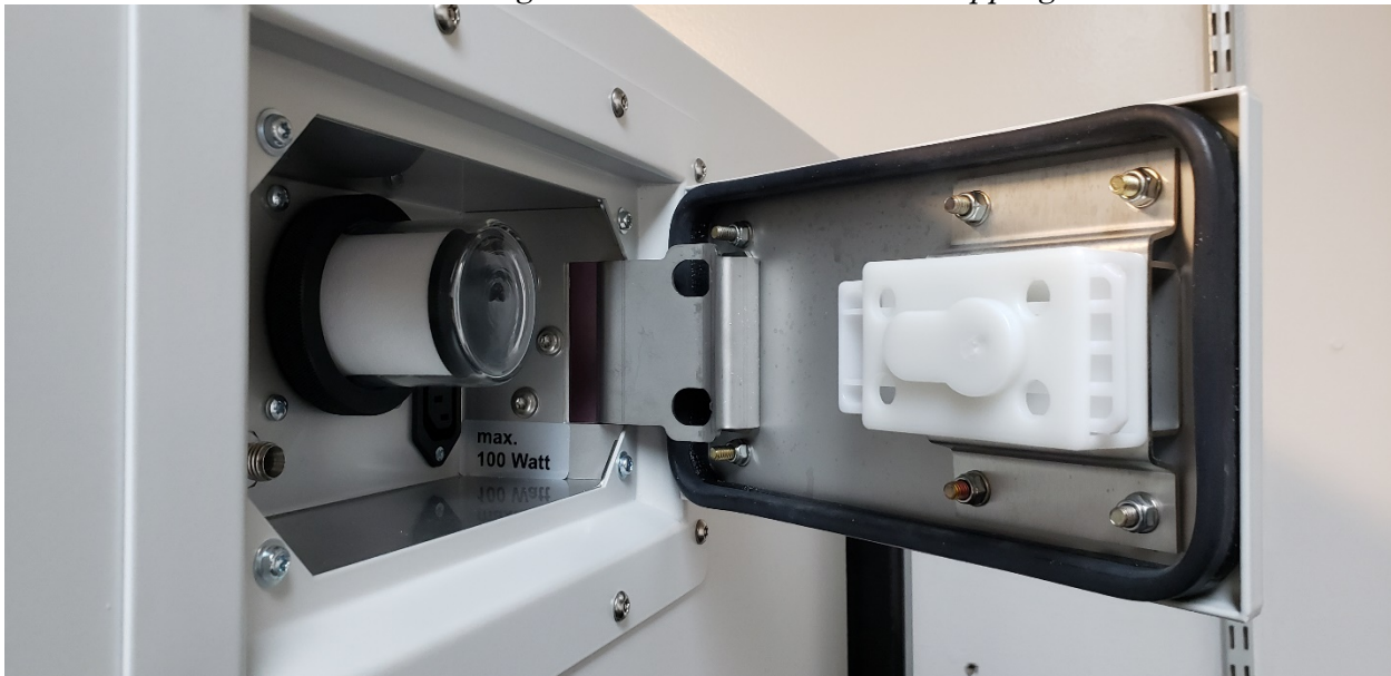
Access Door locking mechanism and weather stripping
