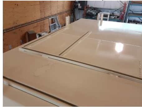
Weld-on uni-strut for roof mounting
