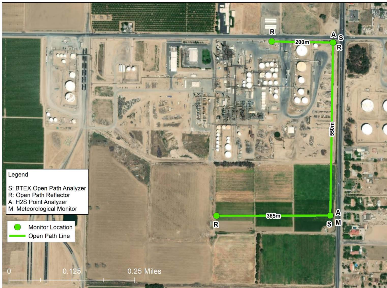
Figure 2. Location of sensors and measurement paths at the Kern Refinery. Each path consists of a transmitter-detector (S) and a retroreflector (R). Point analyzers locations (A) are in the northeast and southeast corners. The meteorology station is also shown (M).
