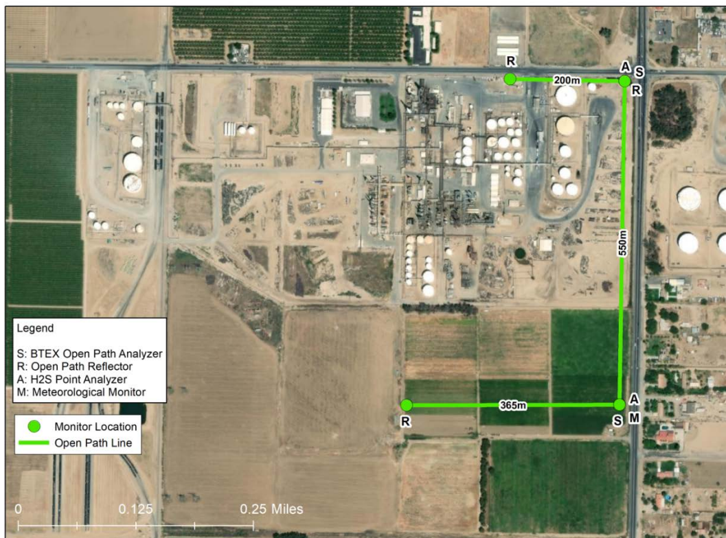
Figure 4. Locations of monitors covering the important fencelines around Kern.
