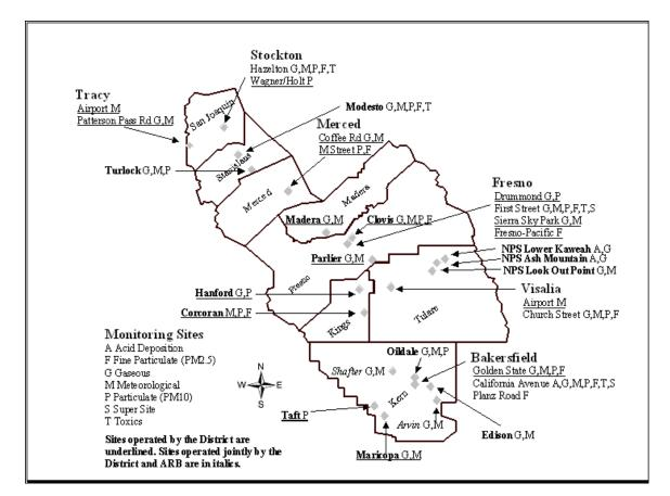
The SJVAB has 23 ozone monitoring stations, with eleven operated by District personnel, three by the National Park Service, and nine by ARB. All ozone monitors are continuous analyzers and operated on the principle of ultraviolet absorption (40 CFR Part 50). Table 2-2 lists all ozone monitoring sites in the SJVAB.
