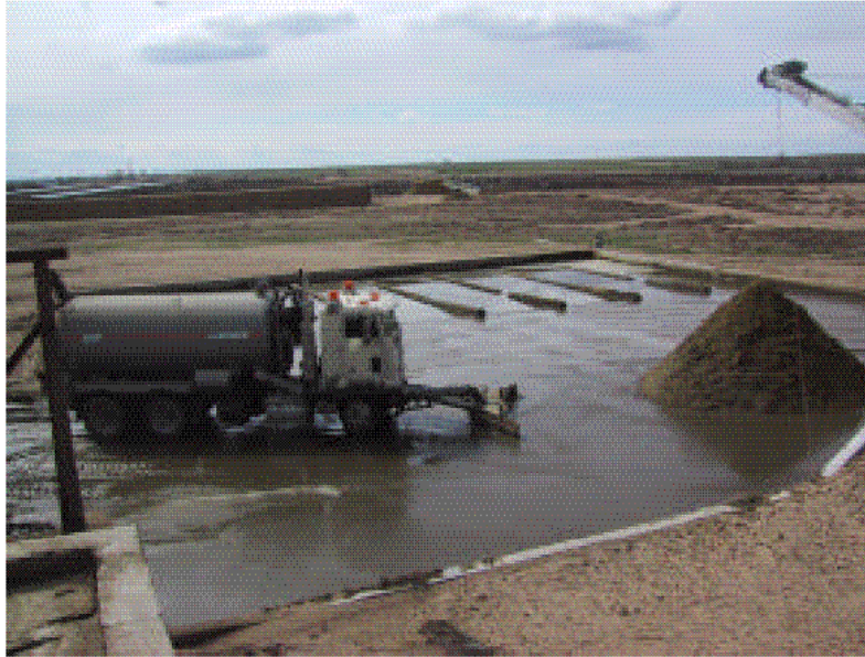
Vacuum Truck Collecting Manure Solids
