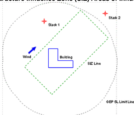
Figure 4.6 -GEP 360° 5L and Structure Influence Zone (SIZ) Areas of Influence (after U.S. EPA(24)).
