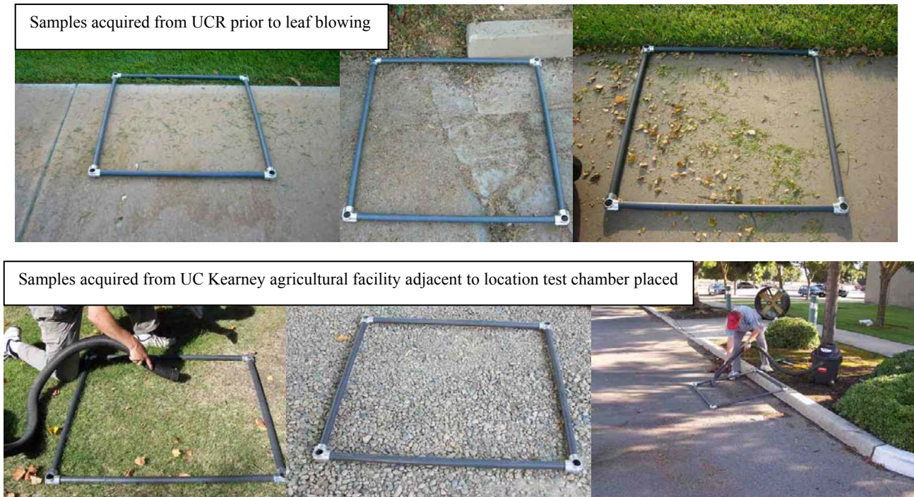
Figure 26. Square meter areas vacuumed and analyzed just prior to leaf blowing.
