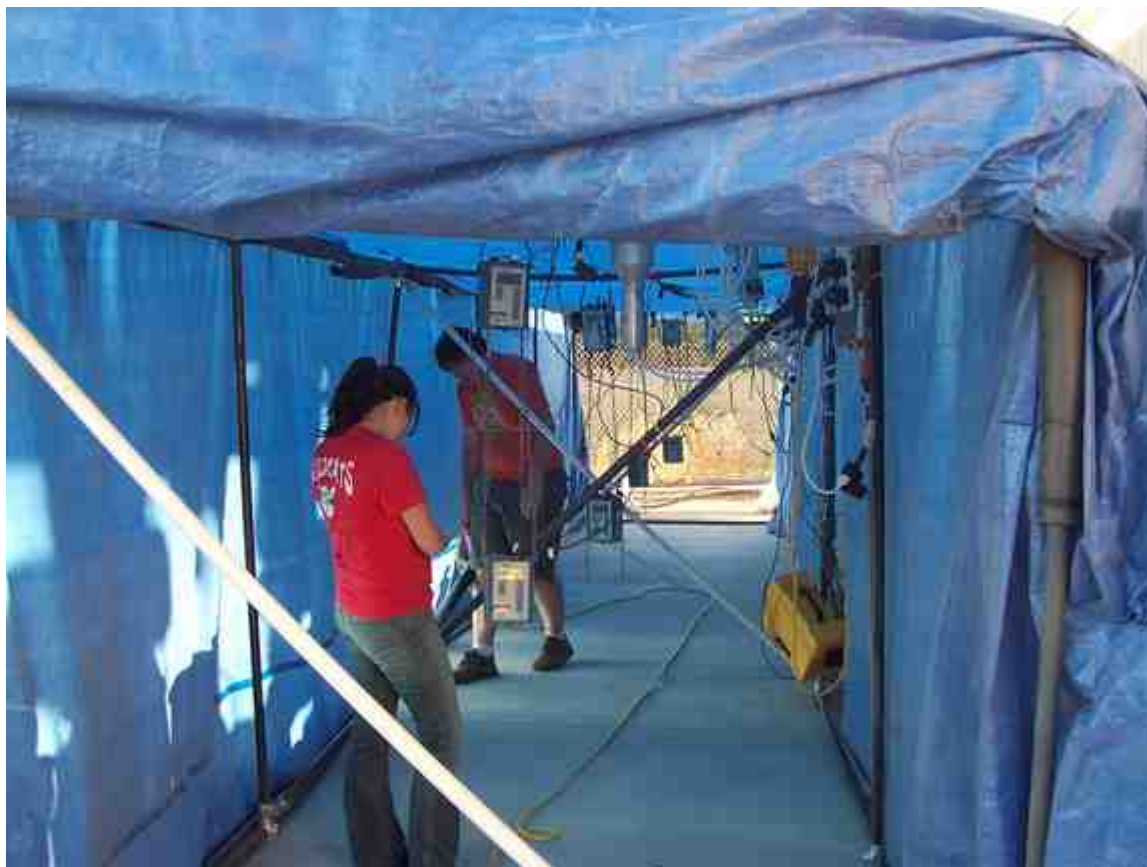
Figure 21. DustTrak locations in 10m test chamber for determining horizontal and vertical particulate matter concentration gradients.
