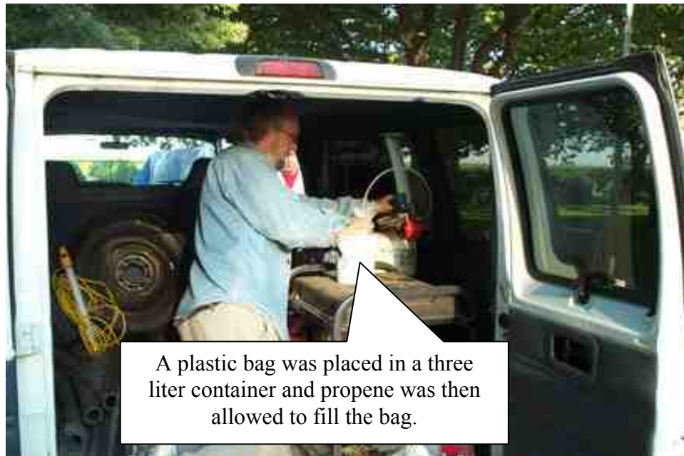
Figure 3. Propene tracer gas preparation.
