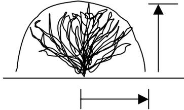
$$\text{Frontal Silhouette Area} = (3.14 \times \text{Maximum Height} \times 1/2 \text{ Maximum Width})/2 \quad \text{Eq. 18}$$
