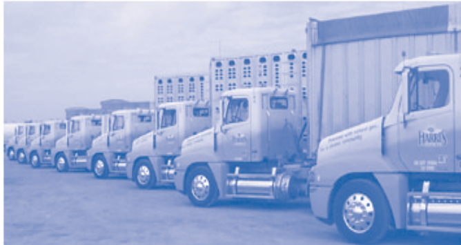
Harris Ranch replaced 12 of its older, diesel trucks with new trucks that burn a mixture of 85% LNG and 15% diesel.
